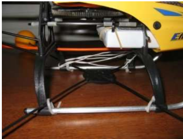
Blade CP training gear mounted on a Blade CP with super skids using zip ties.
