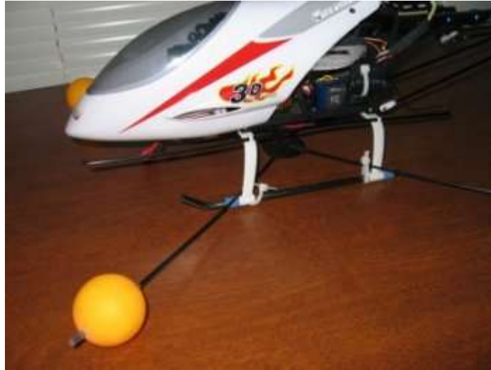
Blade CP training gear mounted on a T-rex using zip ties.
